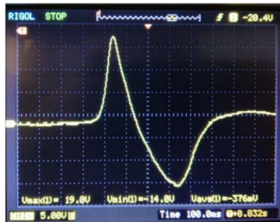
Figure 5. The voltage output waveform for the piezoelectric transducer when placed in a 3D model with 30 mm in diameter
