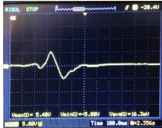
Figure 4. The voltage output waveform for the piezoelectric transducer when placed in a 3D model with 0 mm in diameter
